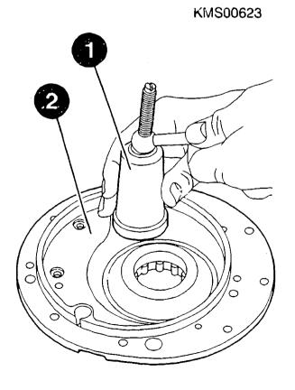
CHECKING/REPAIRING DRIVE AND REDUCTION GEAR END SHIELD
